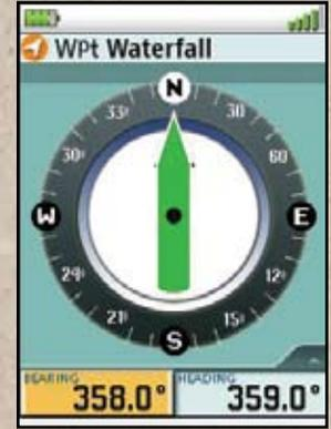
The Triton 2000's 3-axis electronic compass provides precise heading and bearing information.
